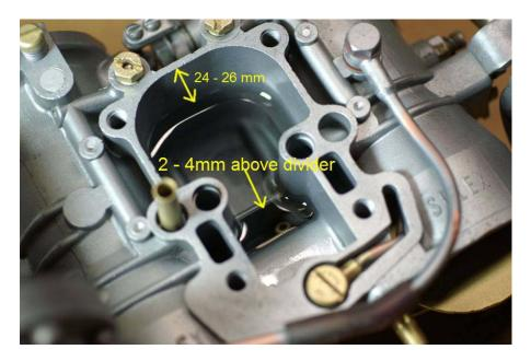
The next step is to check carburetor float levels. Beginning with a cool engine, start and run for 30 - 60 seconds at 1800 rpm.
